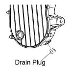
**NOTE:** The sealing surfaces on the drain plug and the oil tank should be clean and free of burrs, nicks or scratches.
